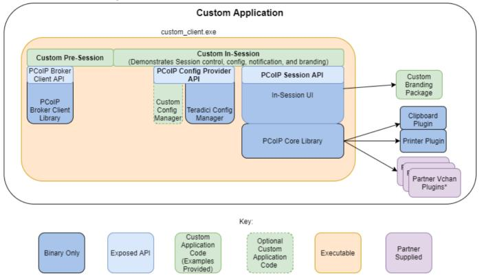
\*Partner Virtual Channel Plugins can be developed using the Virtual Channel SDK, to enable this you can combine the PCoIP Client SDK with the PCoIP Virtual Channel SDK.
